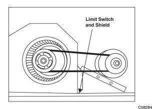
Fig. 28 - Limit Switch Location
